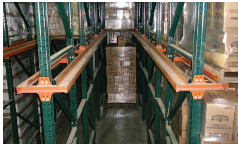
Narrow pallet lanes provide high-density storage.
